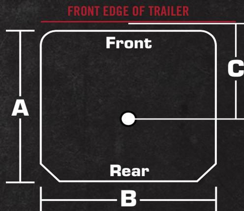
**KP Setback = Measurement from the front edge of the trailer to the center of the king pin.**
