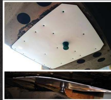
**\*Warning: DO NOT use a Minimizer 5th Wheel Slick Plate, Trailer Slick Plate, Slick Disk, or a Mfg Low Lube 5th Wheel Topplate in conjunction with one another. Doing so could cause a coupling failure. DO NOT INSTALL the Trailer Slick Plate if it extends past the front edge of the trailer or the upper bolster plate.**
