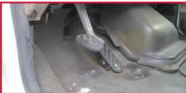
• Kit FKST3B shown in Figure 5 is compatible with 1996-2009 Sterling/Ford Models with floor mounted throttle pedal and floor mounted brake pedal as shown in Figure 6.
