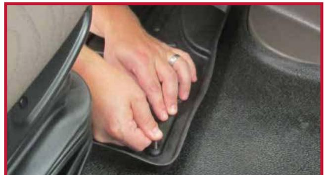
15. Position the passenger floor mat in the truck. Make sure the passenger mat is pushed all the way forward so the outside lip makes full contact with the doghouse trim panels.
