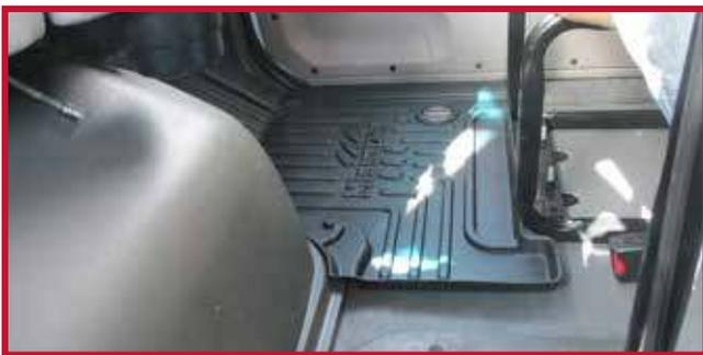
17. Confirm that the retention hook is fully engaged into the driver mat and that the hook is adhered to the floor. If the driver mat hook is not functioning properly or the mat cannot be securely installed, do not use a Minimizer floor mat on the driver side of the vehicle.
