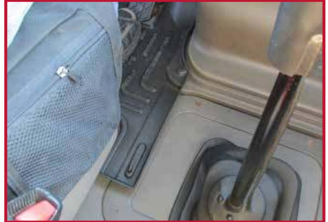
Mark the approximate position where the hook needs to be attached to the floor. Once the position is located, remove the driver mat from the truck.
