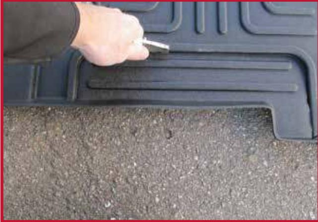
**CAUTION:** Minimizer floor mats are designed to be used with the factory rubber flooring in good condition. If the factory floor is in poor condition (has humps or bubbles) due to excessive moisture, the floor mat may not sit in place properly. If the floor mat does not sit in place properly there is risk that the floor mat will interfere with the brake and throttle pedals.
