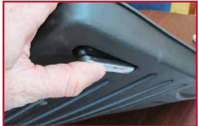
8. Once the hook is in place, let the mat and hook rest on the floor as shown in Figure 6. Next, confirm that the mat is not interfering with foot pedals and verify it is making proper contact with the surfaces surrounding the floor.
