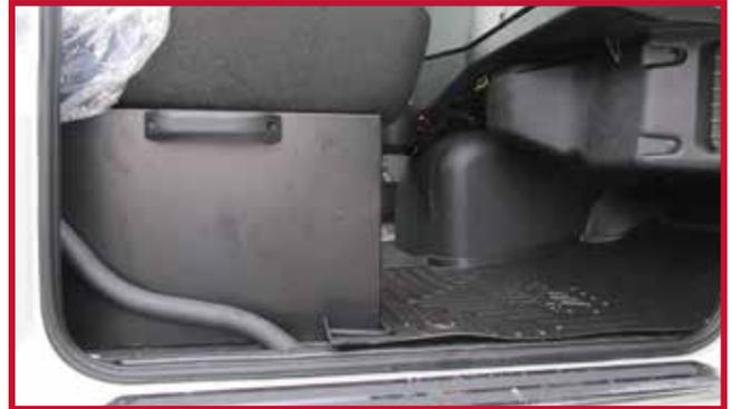
Figure 14 - Fixed Base Passenger Seat with Trimmed Mat
