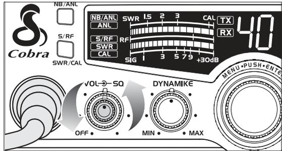
3 To achieve the Desired Squelch Setting (DSS), turn the Squelch control *counterclockwise* until you hear noise. Now turn the control *clockwise* just until the noise stops. This is the DSS setting.
