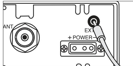
1 Connect an external speaker to the external speaker jack on the rear panel.
