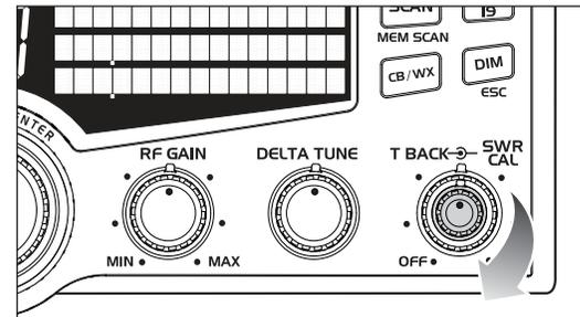
4 While *holding* mic button *adjust* the **SWR CAL** knob so the meter swings to the CAL mark on the meter (located on the right).
