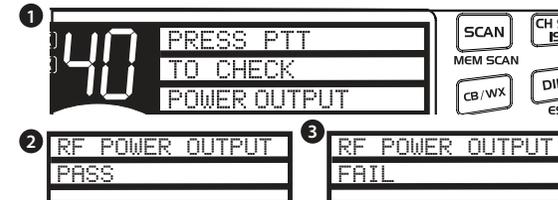
**Test 3- Antenna Mismatch Warning:** Press **Push-to-Talk** button to check antenna/radio for proper matching.
