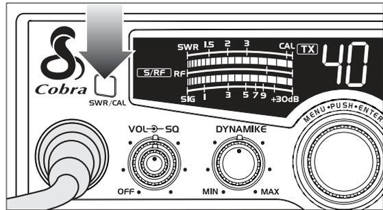
1 The **S/R/F-SWR-CAL** button must be in the S/R/F mode.
