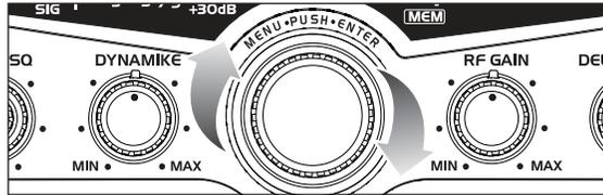
Rotate **Menu/Enter** knob *clockwise* to navigate menu levels.
