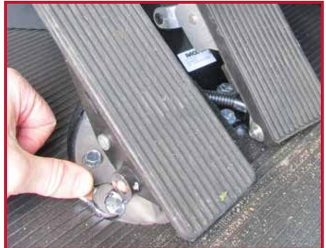
9. Remove the nut from the 5/16-18 x 1" bolt using a 1/2" socket and open end wrench. The nut is accessible on the bottom side of the cab.
