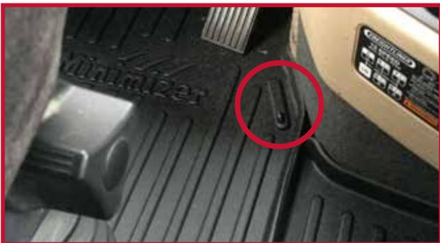
17. Pull the driver mat toward the rear of the truck to confirm that the hook is fully engaged into the mat and that the hook is adhered to the floor. If the hook is not functioning properly or the mat cannot be securely installed, do not use a Minimizer floor mat on the driver side of the vehicle.
