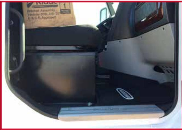
6. Test fit the driver mat in the truck. The driver mat is designed to fit underneath the throttle pedal. To install the driver mat, lift up the heel portion of the throttle pedal and slide the front of the floor mat underneath the pedal. Confirm that the mat is pushed all the way forward so it rests against the fire wall.
