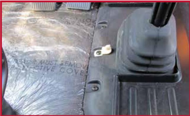
10. Install the driver side floor mat and engage it into the retention hook. The driver mat must be pushed all the way forward so the front lip makes full contact with the lower dashboard kick panels. If installing kit FKP2B or 104104 nest the right edge of the mat over the top of the left hand edge of the passenger mat to lock the floor mats together. If installing kit FKP3B or 104105 nest the left edge of the passenger mat over the top of the driver mat.
