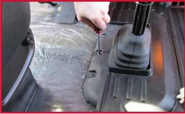
b) Insert the screw through the hole in the retention hook as shown in Figure 12.
