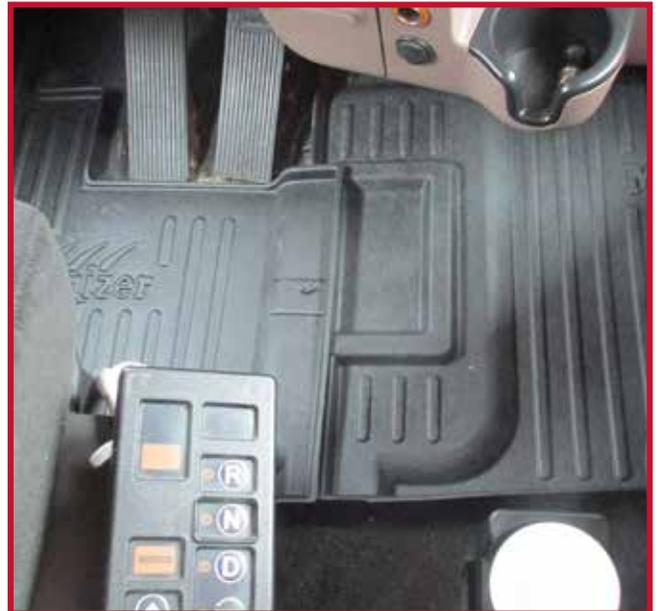
9. Install the retention hook to secure the driver side floor mat from any movement. Follow installation steps a, b, and c below.
