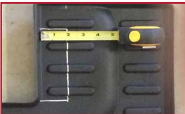
7. For cases where a fire extinguisher is mounted behind the driver seat, the left rear corner of the center mat shaded in yellow may be trimmed to allow for clearance.
