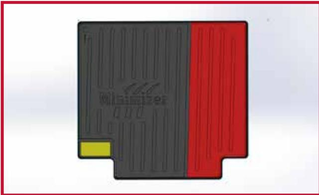
6. Trucks with a 18 speed transmission that are equipped with a MX13 Paccar engine require hand trimming of the passenger mat for proper fit around the gearshift. As shown in Figure 7, draw a line on the floor mat 1.75" away from the inside edge of the front lip around the gearshift. Use a utility knife to trim the floor mat material along the line. After trimming, the mat will lay properly in the truck as shown in Figure 8.
