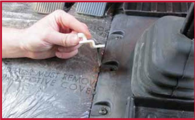
c) Insert the hook through the hole in the transmission cover and tighten using a #3 Phillips screwdriver. Orient the hook so it points straight toward the gearshift as shown in Figure 13.
