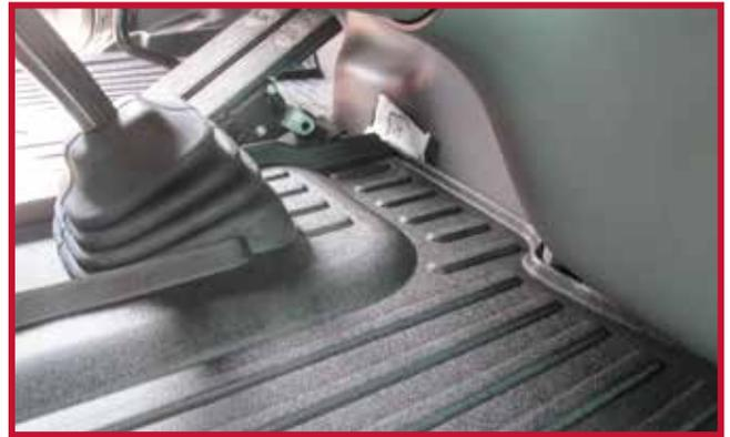
8. Next install the mat for the passenger side of the vehicle as shown in Figure 9.
